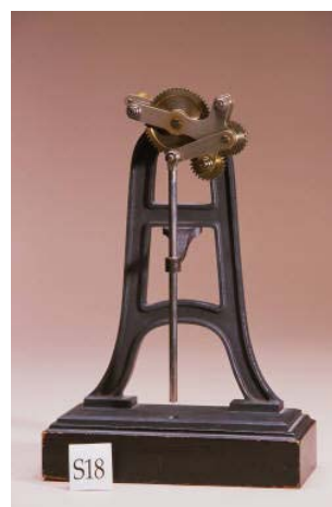
S18 Epicycloid Straight-Line Linkage ii
