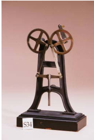
S34 Cartwright Straight-line Mechanism iii
