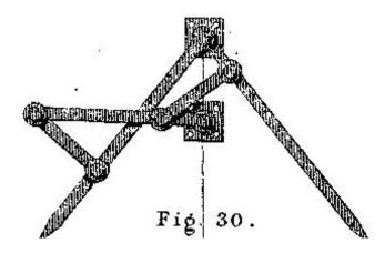
An extension of the linkage employed in these two last figures gives us an apparatus of considerable interest. If I take another linkage contra-parallelogram of half the size of the smaller one and fit it to the smaller exactly as
